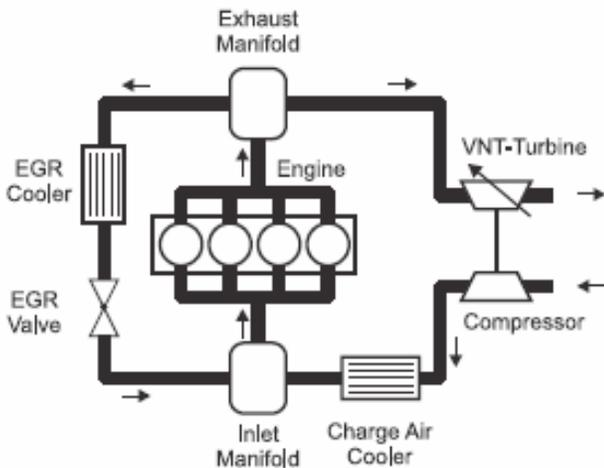
Figure 1. Schematic diagram of a turbocharged diesel engine [7]
