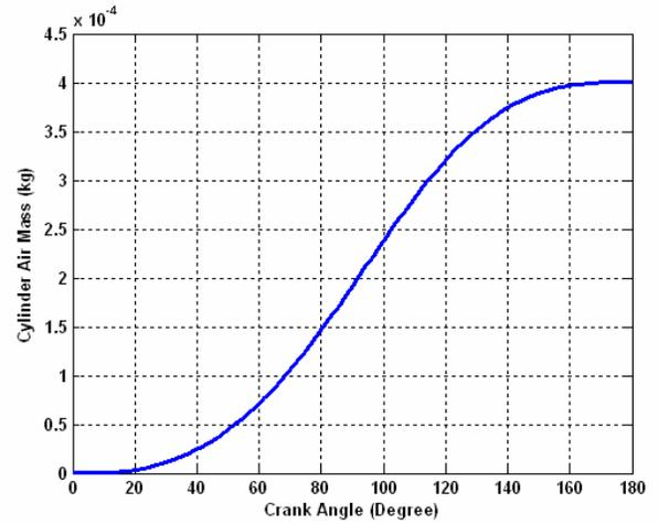
Figure8. Mass of air in the cylinder
