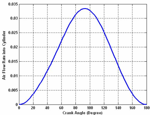
Figure7. Air flow rate into cylinder
