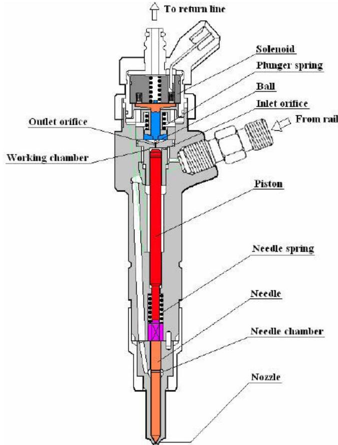
Figure2. Diagram of a Bosch injector [13]
