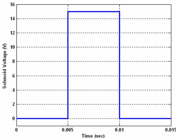
Figure11. Control signal (voltage) of solenoid
