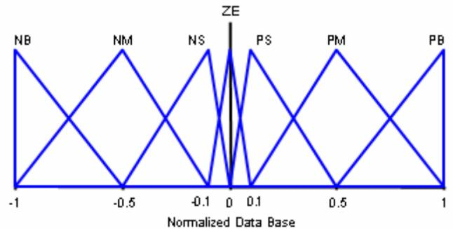
Figure3. Membership Function shape for inputs and output
