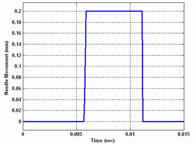
Figure12. Needle movement
