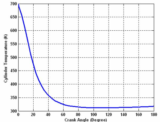
Figure9. Cylinder temperature variations
