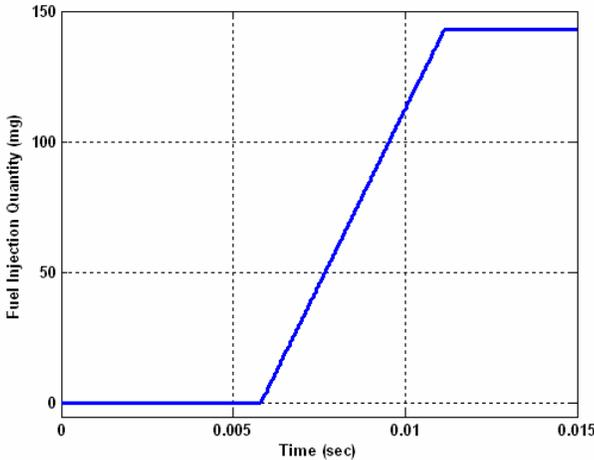
Figure14. Injection quantity in one injection duration
