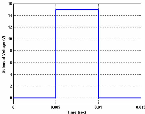
Figure11. Control signal (voltage) of solenoid
